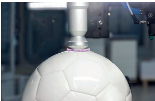
Fig. 4. Polyurethane: treatment with Openair-Plasma makes it possible to achieve permanent printed images on objects exposed to high mechanical stress © Plasmamatreat
