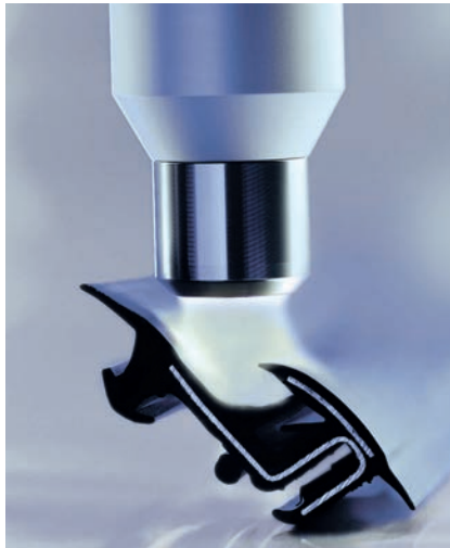
Fig. 3. EPDM: surface treatment activates this non-polar material for vehicle door and window seals and prepares for subsequent coating in a faster and, above all, cleaner process © Plasmamatreat
