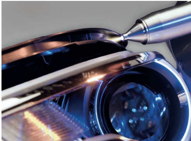
Fig. 1. Polypropylene: in fitting the lenses on car headlight housings, Openair-Plasma pretreatment ensures reliable bonding and a tight seal © Plasmatrete
