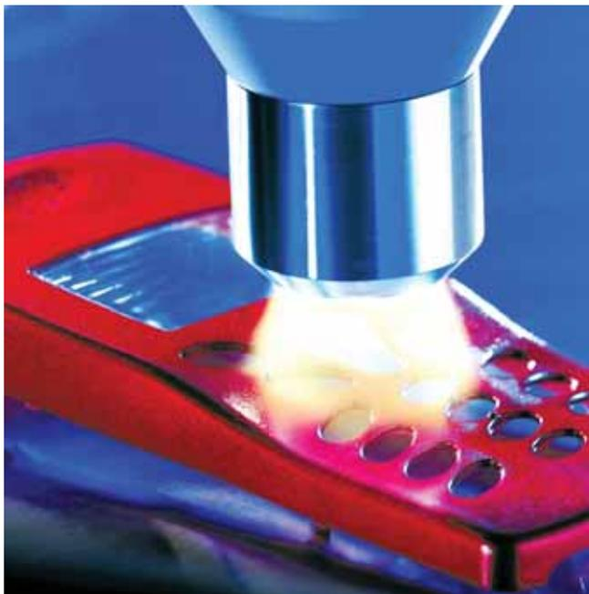
**Windows can be glued into place in the housing shells of mobile phones using atmospheric plasma polycarbonate and solvent-free UV adhesives.**
