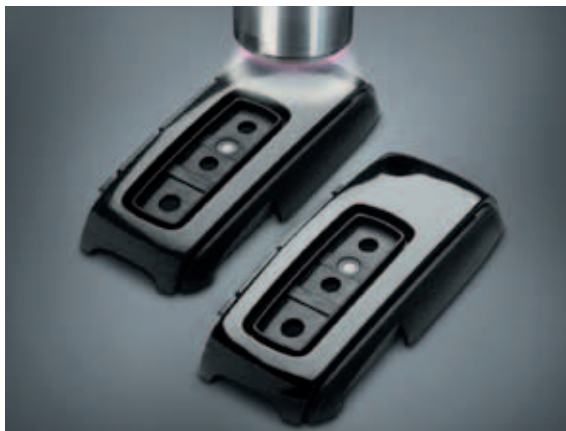
FIGURE 3 | The left shows the pretreatment of the key's bottom shell with Openair plasma. The right is the same part after application of the transparent scratch-resistant coating.
