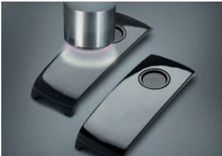
FIGURE 1 | The polyamide shells of a key design are pretreated with atmospheric plasma.
